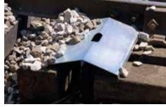
Four Ballast Shields to protect the lifting cylinders.
