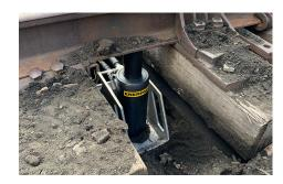
Four framed lifting cylinders, each rated for 62 tons, offering a total lifting capacity of 248 tons.
