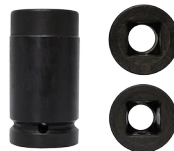
08-3410 SOCKET, 1 DRIVE, 15/16 BROACH, 4 PT. (FOR TIMBER SCREWS)
